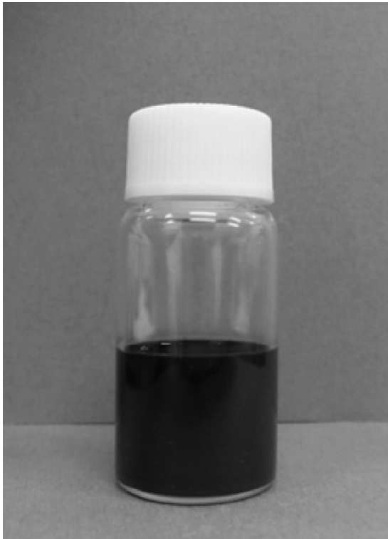
Fig. 3. LSCF–GDC ink after sedimentation test lasting 1 month.
